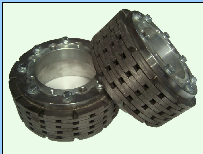
“PACK RINGS” CALIBRATING ROLLERS MC8 ON ROTATING HEADS. (no.8 wheels for each head).
